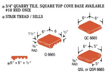
\* Q 6665 series is a lip bullnose for concealing setting bed. In combination with standard tile and cove base units, there is unlimited flexibility for sill, stair tread and riser dimensions.
